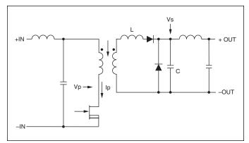
**Figure 9–6** — Basic zero-current-switching converter topology (VI-200 / VI-J00)
